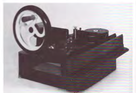
NPM 91/7 Hand-operated Krag 'Continuous Impression' cancelling machine. Developed in Norway this simple but efficient machine was introduced into Great Britain in 1907 after trials in London. (NPM Collection)
