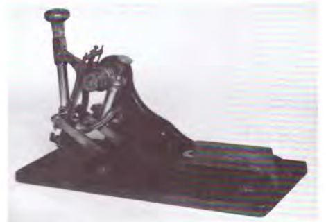
NPM 91/7 Hand-operated Krag 'Continuous Impression' cancelling machine. Developed in Norway this simple but efficient machine was introduced into Great Britain in 1907 after trials in London. (NPM Collection)
